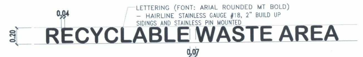
TYPICAL ROOM SIGNAGE DETAIL SCALE: 1:25 METERS
