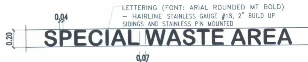
TYPICAL ROOM SIGNAGE DETAIL SCALE: 1:30 METERS
